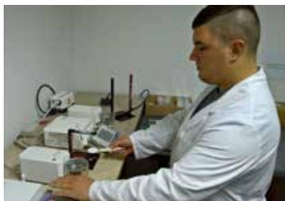
Particle matter sample weighing
